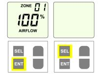
Press the Up or Down key to change the Address number then press the ENT key to save the change. Use the Up or Down key to adjust the airflow then press the ENT key to save the change.
