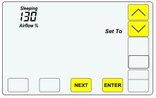
The Sleeping Airflow% is displayed. Press or to adjust the amount of heating or cooling to the upstairs sleeping zone. Press ENTER to save the new airflow setting. The upstairs temperature (Sleeping) is displayed and used to control heating and cooling calls.
